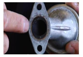
2. If you are reusing the emission valve, clean the exhaust side with carb cleaner and brush. Ensure the valve does not leak and that it opens in the direction of flow by blowing through it.
