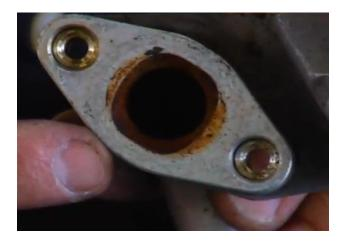
3. Clean aluminum tube from both sides with hand brush and carb cleaner until tube is clean, bend brush as needed. Note: After using the brush to clean the pipe out you will see how the carbon is removed from both ends and the part is much cleaner.
