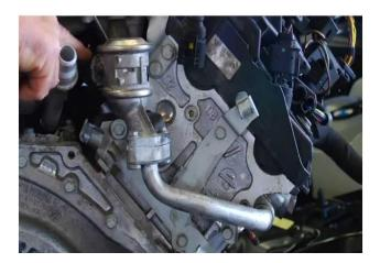
1. Remove emission control valve on the side/sides where you want to perform the cleaning. The plastic tube tends to stick to the valve, take care not to break the plastic tube during removal. Note: If your vehicle has over 100,000 miles as a rule we recommend replacing the valve during the cleaning because the diaphragm gets stiff and will also restrict the airflow into the cylinder head.
