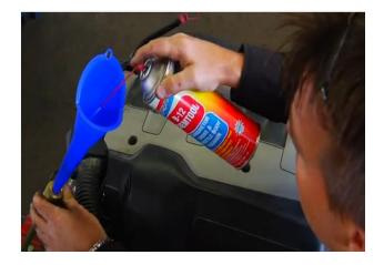
5. Insert funnel and fill with cleaner. On some cars the cleaner will sit in funnel, this depends on how plugged the system is. Repeat this step 2-3 times and allow cleaner to sit approx. 20-30 minutes each time.
