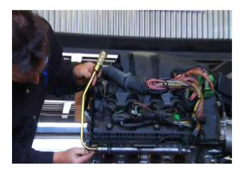
4. Clean hole in back of cylinder head. Insert tube in hole so O-ring is making a seal.
