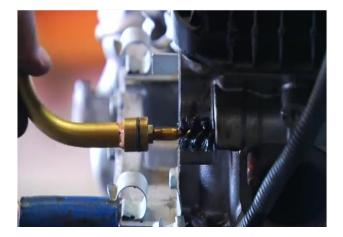
**Note:** Run drill clockwise ONLY. Counter clockwise can cause brush to loosen and fall off. Start cleaning passage; the funnel will help guide the cable.
